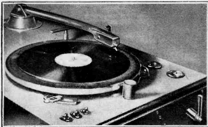
A NEAT IDEA from Radio Geneva, photographed by our Swiss Correspondent. With the help of the transverse guide bar on which the pick-up arm rests, the needle may be placed accurately above any desired groove of the record. The pick-up is then lowered on to the record by means of the lever in the lower right-hand corner of the photograph.
