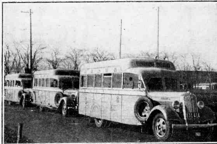
TELEVISION IN TOKIO. Dr. Kenjiro Tagayanagi conducted the first television O.B. in Japan on February 11th, when scenes of the national celebrations were transmitted by the new mobile unit shown above.
